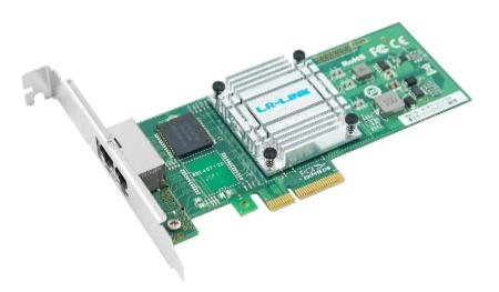
LRES2024PT is a PCI Express v2.1 x4 dual-port Gigabit Ethernet network adapter developed by Shenzhen Lianrui Electronics Co., Ltd. based on the WX1860A2 solution of the domestic main controller WebEx Technology. This adapter is compatible with PCIe x4, x8 and x16 and backward compatible with PCIe v1.1. The adapter card achieves a dual-port bidirectional communication transfer rate of 4GB on a PCI Express v2.1 x4 bus.
