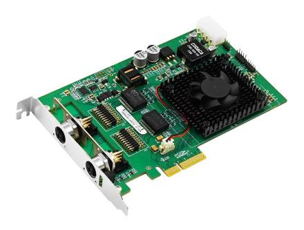
LRES4013M-POE is a PCle3.0 x4 dual-port M12 interface 10G ethernet image acquisition card independently developed by Shenzhen Lianrui Electronics Co., Ltd. (abbreviation: LR-LINK) based on the Intel X550 main control solution. Image acquisition card, cit is compatible with PCle x8, x16. The network card is mainly designed for industrial field visual inspection equipment, visual field client, fast mobile Ethernet data transmission equipment, field monitoring, industrial monitoring, etc.
