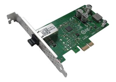
LRES2001PT-POE is a PCIe x1 PoE+ gigabit single-port copper industrial ethernet network adapter based on the Intel chipset be developed independently by Shenzhen Lianrui Electronics Co., Ltd and is compatible with x4, x8, x16. The adapter is designed mainly used on industrial field vision inspection server and equipment, vision field client, fast moving ethernet data transmission equipment etc. It's also suitable for ordinary servers.
